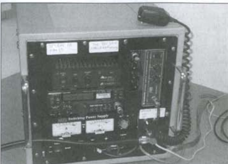
N7BHC 2m beacon rack
